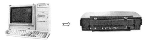
In this situation, the card will have a built-in terminator. The card forms one end of the SCSI chain, the scanner forms the other end. Simply turning on the *active terminator* of your scanner.
